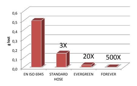
When tested in accordance with ISO 6945 specification, EVERGREEN rubber cover shows abrasion resistance up to 20 times better results
